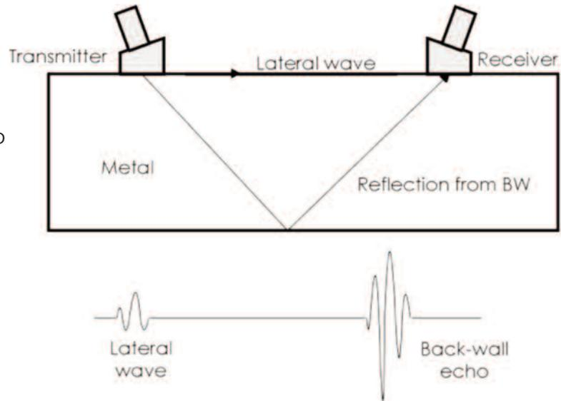
Figure 2: TOFD principle
