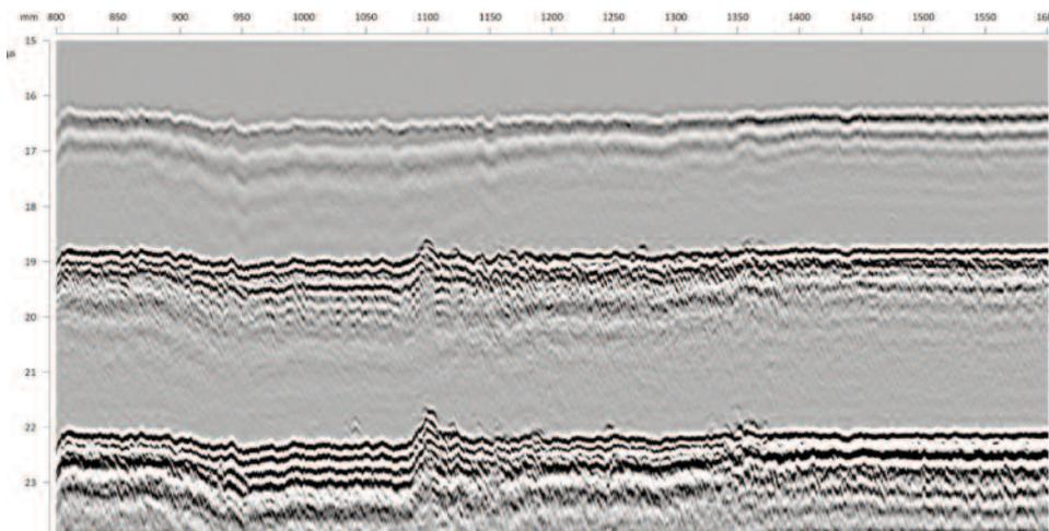
Figure 3: TOFD scan showing corrosion
