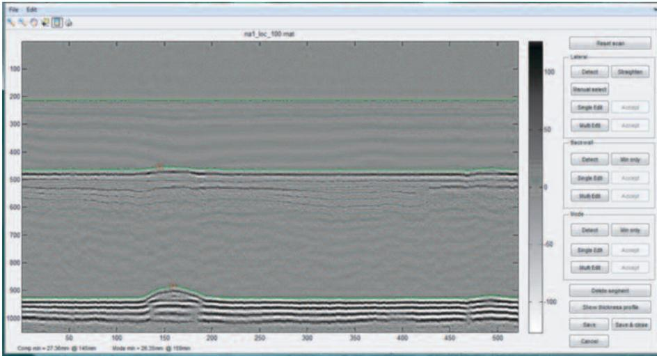
Figure 4: TOFD scan after processing in Sonomatic's bespoke software
