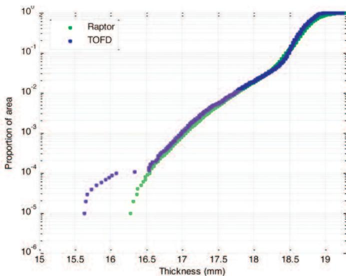
Figure 7: Cumulative thickness distributions for zero degree corrosion mapping (Raptor) and TOFD
