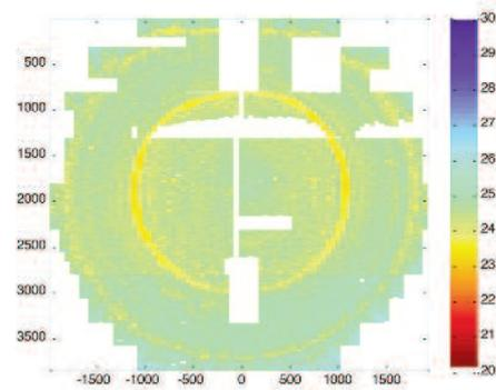
Figure 5: Corrosion map generated from TOFD data of dome end
